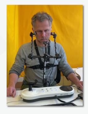
The instrument's chord panel can be rotated up to 180 degrees, allowing for countless ways to hold the instrument, which can be hugely helpful for musicians who feel more comfortable using their heads, toes or elbows than their fingers.
